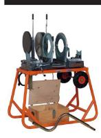
A professional welding machine ideal for medium sized pipes and sewers up to 315mm. The MAXI315 can weld fittings such as bends and tees. Branches can also be welded thanks to the single clamps (available on request) indicated for all diameters in the working range. Available in 110 V and 230 V
