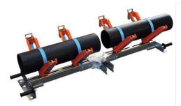
An essential and professional tool for the alignment and support of pipes during electrofusion from Ø 125mm to 500mm (4" IPS ÷ 20" IPS). The ALIGNER is entirely made of steel, featuring a central adjustable joint and pipe fastening clamps fixed on axes.
