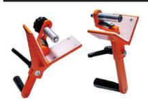
These are professional tools for beveling the ends of plastic pipes up to 315mm, which will be inserted into electrical couplers or plug-in joints.
