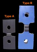
**Result samples**Left: Brittle failure
