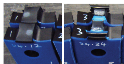
Result samples Left: Brittle failure Right: ductile failure
