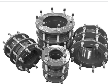
Fully Restrained Dismantling Joint AS 4087, PN16 316 SS Rods
