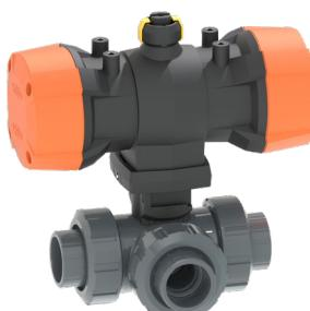
The 285-288 model incorporates the +GF+ 543 3-Way Bal Valve and a compact pneumatic actuator available in either L or T-Port configuration. The L-Port configuration normally requires a 2 position 90 degree actuator whilst the T-Port valve may require a 3 position Electric Actuator. Available Fail Safe Close, Fail Safe Open or Double Acting. A visual position indicator shows valve position. Please contact us for the valve material and the actuator configuration you require.
