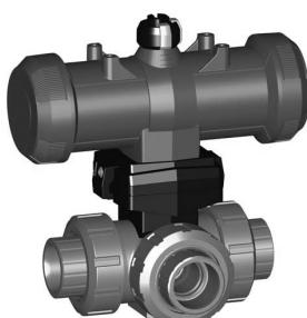
The 285-288 model incorporates the +GF+ 543 3-Way Bal Valve and a compact pneumatic actuator available in either L or T-Port configuration. The L-Port configuration normally requires a 2 position 90 degree actuator whilst the T-Port valve may require a 3 position Electric Actuator. Available Fail Safe Close, Fail Safe Open or Double Acting. A visual position indicator shows valve position. Please contact us for the valve material and the actuator configuration you require.
