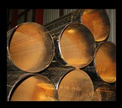
Electric resistance welded (ERW) pipe is fabricated by cold-forming a sheet of steel into a round and hollow shape. Current is passed between the two edges of the steel to warm the steel to a point at which the edges are constrained together to make a bond without the utilize of welding filler fabric.
